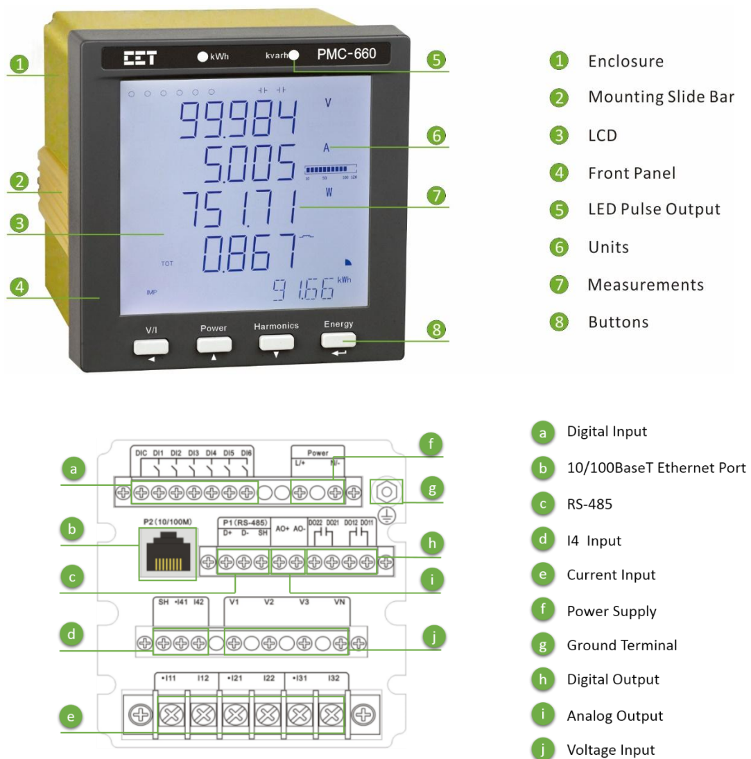
Figure 2-1 Appearance (RS485+6DIs+2DOs+AO)
